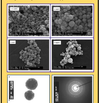
SEM and TEM images of TiO<sub>2</sub> particles with the corresponding SAED pattern.
