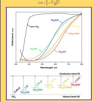
The effective band gap energies of TiO<sub>2</sub>/L (L=CAT, DOP, AA, 2.3DHN and ANT) particles were calculated *by Kubelka-Munk function* to be 1.82, 1.75, 1.72, 1.72, 1.72, and 1.67 eV, respectively. Red shift in reflection spectra is observed in comparison to the bare TiO<sub>2</sub> particles, Eg  $\sim$ 3.18eV.
