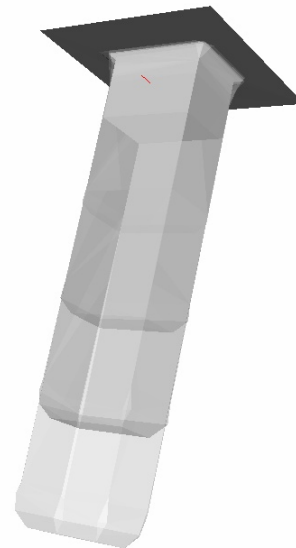
Fig. 2. Optimized Lax-Friedrichs scheme - etching profiles for V = V_0 \cos \theta at t = 0 , t = 30 s, t = 60 s, t = 90 s and t = 120 s.
