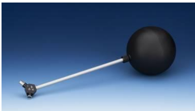
Figure 1. HS01 S/N 112, Secondary standard chamber for H^*(10) (Photo credit Bildstelle PTB).
