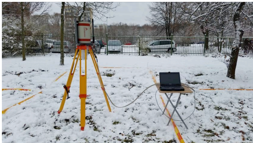
Picture 2. In situ gamma spectrometry measurement
