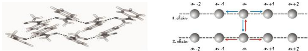
Figure 1. The real structure of the part of crystalline acetanilide macromolecular chains is shown in the left, whereas its schematic structure is demonstrated in the right. The possible vibron hopping transitions are shown by the arrows.
