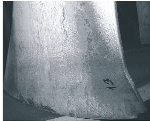
Figure 7. Blade surface with attached layer of dirt
