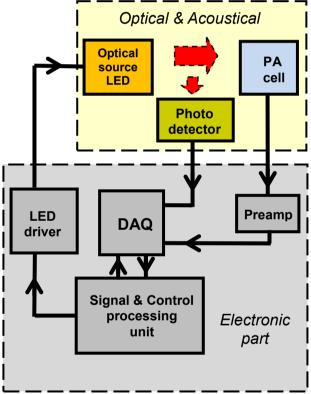
Fig 1.The experimental set-up for PA time-domain measurements.
