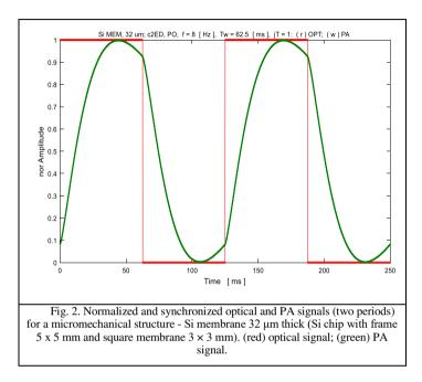
Experimental signals, optical excitation and PA response (in Fig.2 given as the rectangle pulse train and the periodicgreen line, respectively,) have been measured versus as the function of time. Each experimental signal is obtained as the averaged result of at least three measurements. Optical and PA signals are normalized by the following formula:
