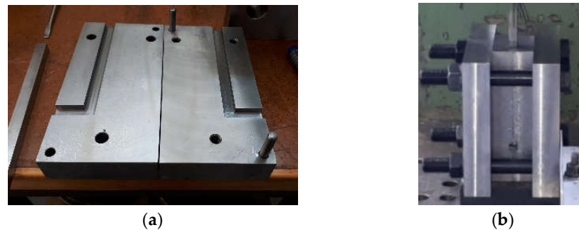
Figure 3. ECAP tool: (a) die and (b) in process.
