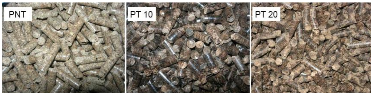
Figure 2. Images of the pellet samples (PNT - pellets produced from non-treated beech particles. PT10 and PT20 - pellets produced from treated beech particles with ~10 and 20 % water content, respectively)
