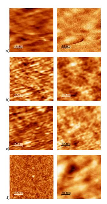
Figure 1: (a-d) Topography(AFM) images (left) and MFM images (right) of Co/Si bilayers: (a) as deposited; (b) irradiated to  $5 \times 10^{15}$  ion/cm<sup>2</sup>; (c)  $10 \times 10^{15}$  ion/cm<sup>2</sup> and (d)  $15 \times 10^{15}$  ion/cm<sup>2</sup>.
