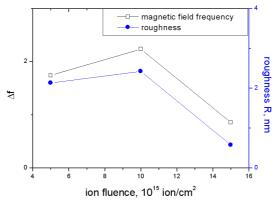
Figure 2: The Xe ion fluence dependence of magnetic frequency ( $\Delta f$ ) and roughness (R) of Co/Si bilayers irradiated with  $5 \times 10^{15}$  ion/cm<sup>2</sup>,  $10 \times 10^{15}$  ion/cm<sup>2</sup> and  $15 \times 10^{15}$  ion/cm<sup>2</sup>.
