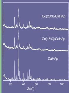
XRD measurements showed pure apatite phase in all samples. By increasing of cobalt amount in CaHAp samples diffraction maximums are shifted to larger angles, also, unit cell parameters decrease.
