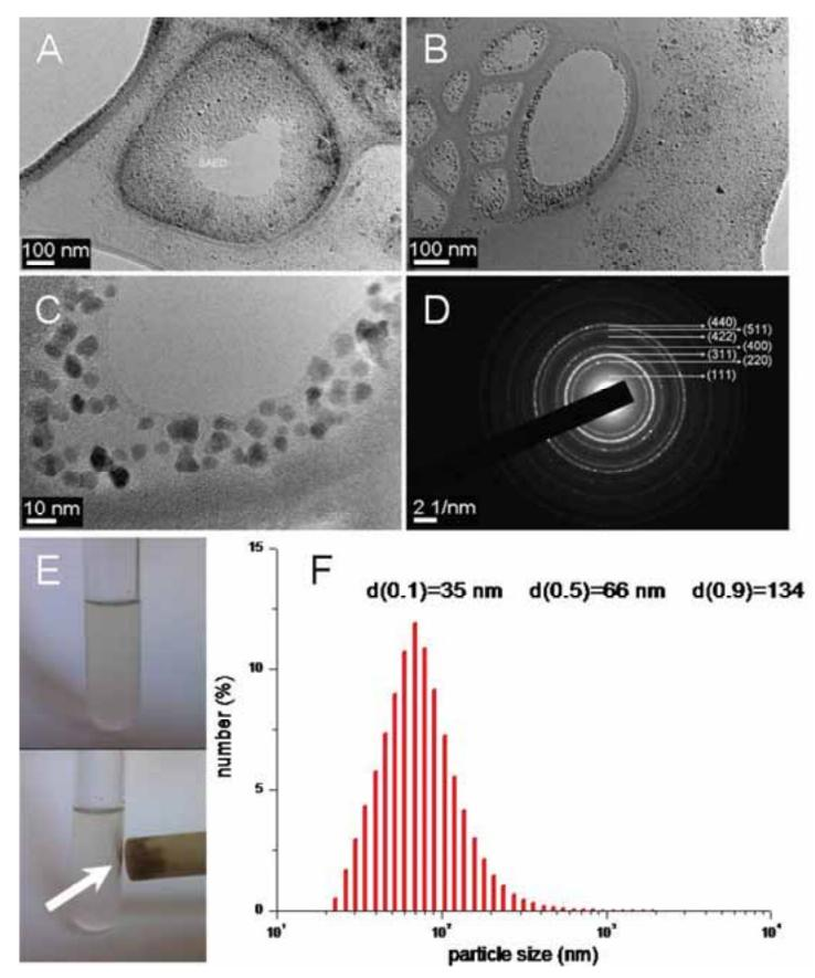
**Figure 6.** TEM images of magnetic nanocrystals immobilized within the poly-(L-lactide) polymer from water dispersions (A, B and C), and SAED of particles (D). The water dispersion of PLA-PEI/MNp stabilized with PVA attracted with a low energy magnet (E) and the size distribution of such hybrid particles measured immediately after sonication (F).
