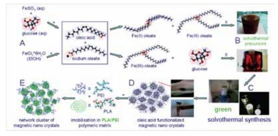
**Figure 1.** Procedures for the preparation of iron oxide magnetic nanocrystals starting from two different precursor salts (A), appearance of solvothermal precursors (B), 100 ml autoclave and the heating set-up used for solvothermal synthesis (C), nanocrystals functionalized with oleic acid, images of dry powder and nanocrystals re-dispersed in chloroform attracted by magnet (D). The magnetic nanocrystals are arranged in 3D network clusters (E).
