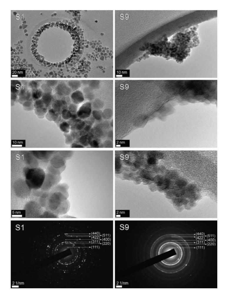
Figure 3. TEM images and SAED patterns of the sample S1, obtained from ferrous sulfate as the precursor salt, and S9, obtained from ferric chloride as the precursor salt.
