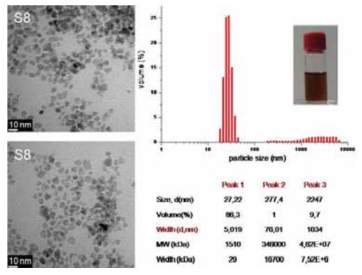
**Figure 4.** Representative TEM images of the sample S8. Particle size distribution and data obtained by DLS measurement of sample S8. DLS data are presented as mean values of three independent measurements (each with five replicates).
