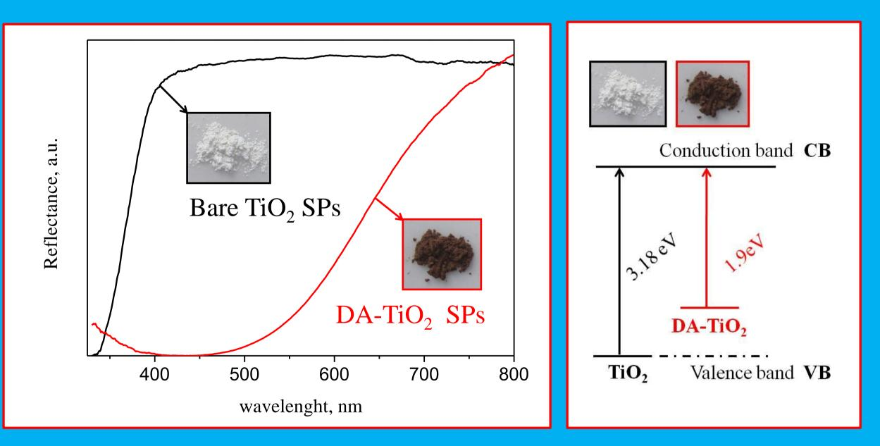
Absorption spectra of colloidal TiO<sub>2</sub> NPs and DA-TiO<sub>2</sub> NPs solutions used as precursors for synthesis of DA-TiO<sub>2</sub> SPs demonstrates red shift of ~1.3 eV indicating formation of the CT complex.
