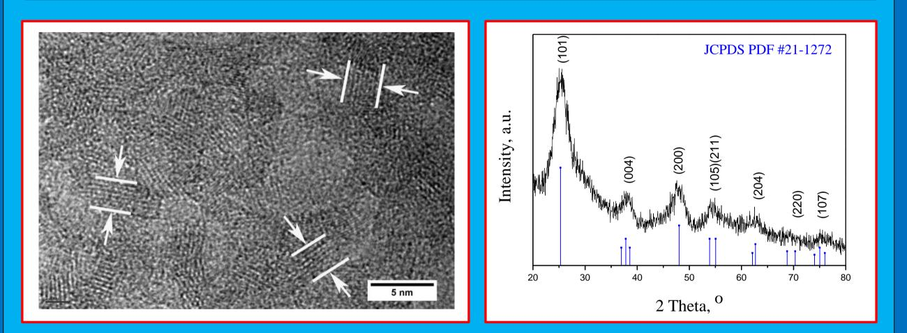
High magnification TEM image of TiO<sub>2</sub> NPs indicates that dry colloidal particles have nearly spherical shape with an average diameter of ~ 4.5 nm. Their XRPD analysis implicates that all diffraction peaks could be assigned to the anatase phase. Low crystallinity is noticeable from the XRPD reflections broadening.
