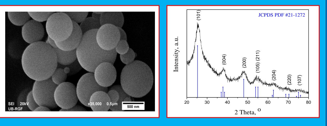
SEM image of DA-TiO<sub>2</sub> SPs shows that obtained particles are spherical in shape and non-agglomerated. Particle mean size is ~ 430 nm, and their composition stay unchanged, i.e. all XRPD reflections belongs to the anatase.
