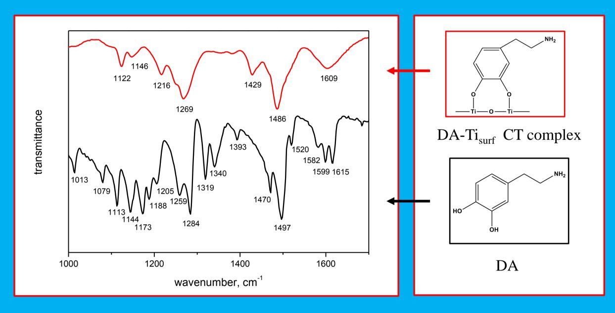
Presented FT-IR results related to the pure DA and DA-TiO<sub>2</sub> SPs agree well with the conclusion made from the Job's curve implicating that determined stoichiometric ratio (2:1) for the complexation of Ti<sub>surf</sub> atoms and DA in DA-TiO<sub>2</sub> NPs stays unchanged in DA-TiO<sub>2</sub> SPs samples.
