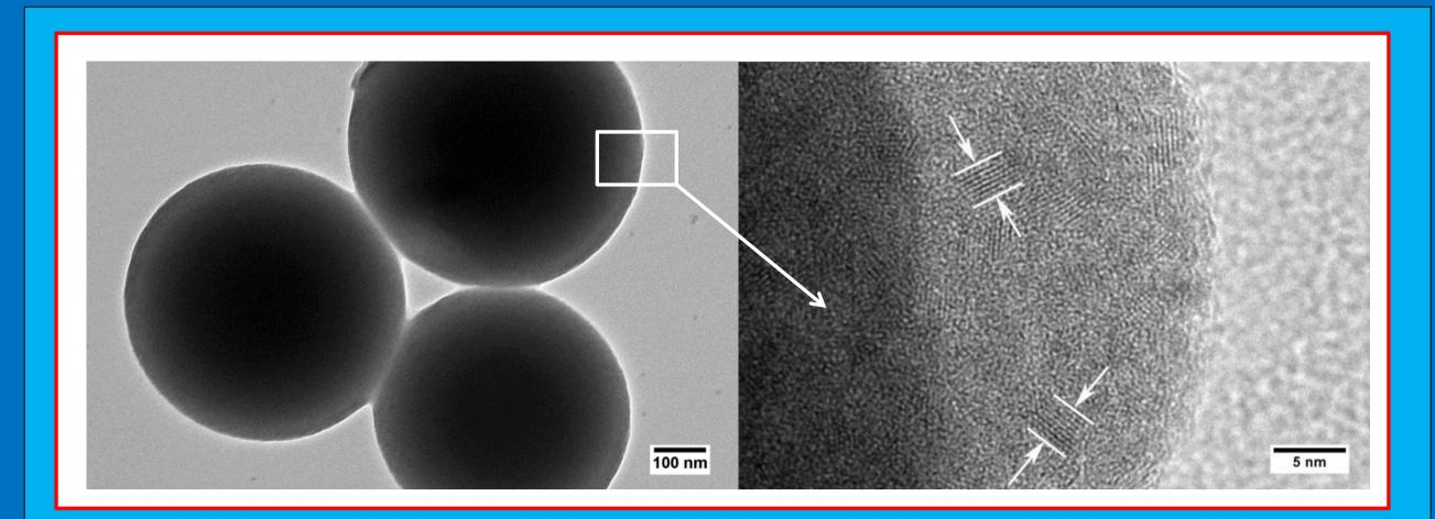
TEM image of the DA-TiO<sub>2</sub> SPs obtained through low temperature aerosolassisted processing of DA-TiO<sub>2</sub> NPs confirms their spherical morphology.
