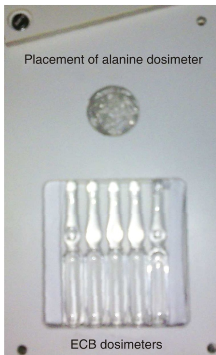
Figure 1. HDRL irradiation phantom showing positions of alanine pellet and ECB ampoules
