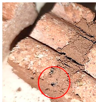
Figure 5. Sample GC 10 applied between ceramic bricks after thermal cycling, with larger waste particles on the surface indicating insufficient homogeneity.
