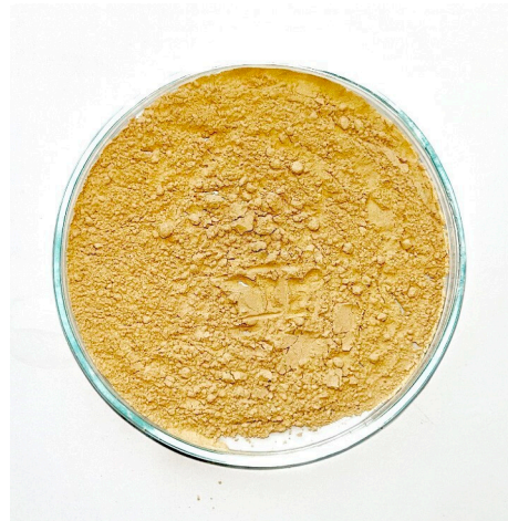
Figure 1. Sample of waste sludge obtained from the wastewater treatment plants.
