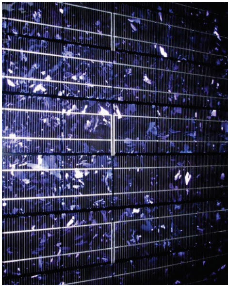
Figure 13. Micro-shading caused by the string connectors
