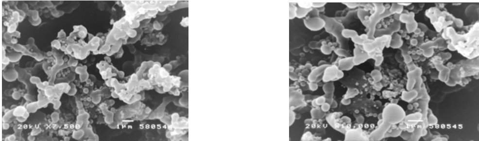
Figure 3. SEM micrographs of particles of biphasic calcium phosphate covered by polymer poly-lactide-co-glycolide
