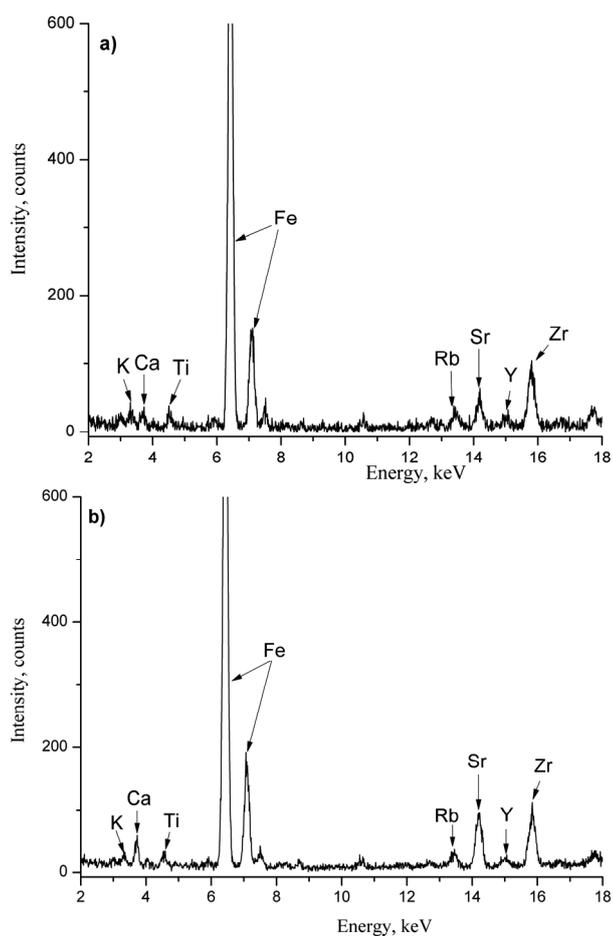
Fig. 6. Representative XRF spectra obtained directly on pottery shards: a) sample P-3, red decoration; b) sample P-4, black decoration.
