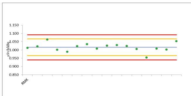
Fig. 1. Unified Sheward chart for 3 RMK 10 type of ambient dose equivalent rate monitors
