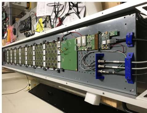
Figure 5.28. The first prototype of a long slab of the SiECAL.
