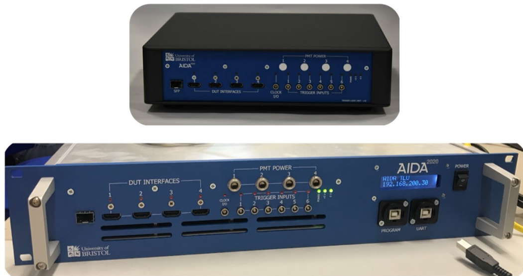
Figure 6.45. The AIDA-2020 newly developed Trigger Logic Unit. Top: table top enclosure. Bottom: 19-inch rack-mounted enclosure. The two enclosures have identical inner components and provide the same functionalities.
