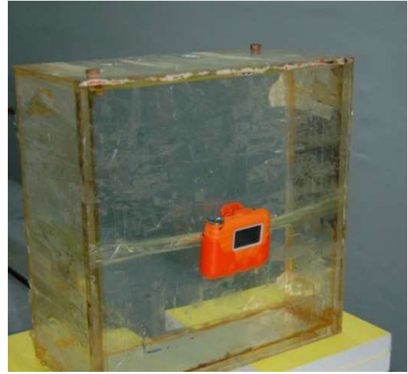
Fig. 2. A PM1610B EPD placed on the ISO water slab phantom prior to the irradiation.
