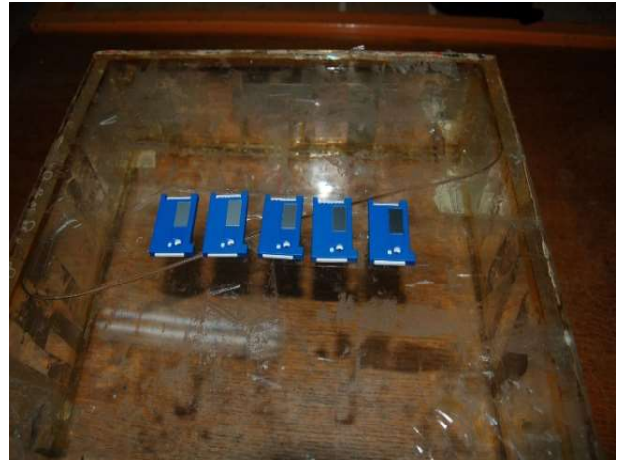
Fig. 1. Five MTS-N TLDS placed on a ISO water slab phantom prior to the irradiation.
