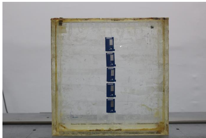
Fig. 1. Five MCP-N dosimeters mounted on the ISO water slab phantom prior to the irradiation.
